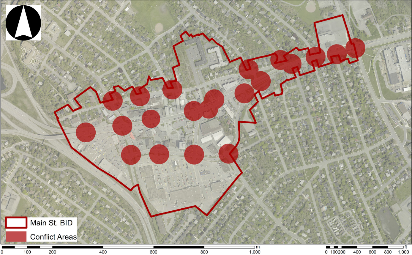
Figure 17: Potential Pedestrian-Vehicle Conflict Areas Image Source: Map by Tim Davidson; Aerial Photography from HRM Corporate Dataset, 2014 (HRM, 2014b); Conflict zones based on site observations)
